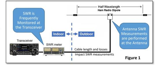
avoids the effects of transmission line loss which can seriously impact measurements. It also eliminates errors introduced by cable length since accurate antenna SWR readings can only be achieved at cable lengths which are a multiple of one-half wavelength.
